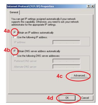
Select: Obtain an IP address automatically (4a) and Obtain DNS server address automatically (4b).
