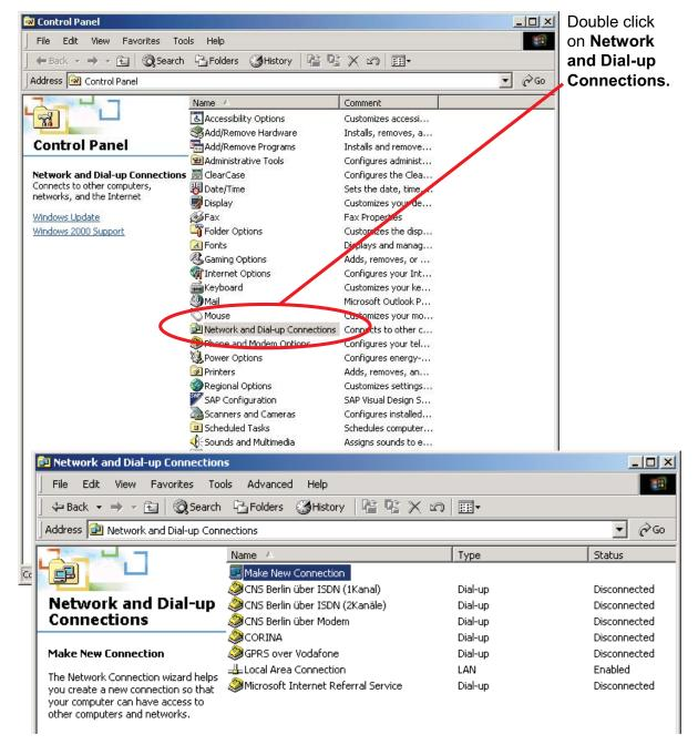
Select **Make New Connection** in order to set up a new dial-up connection.
