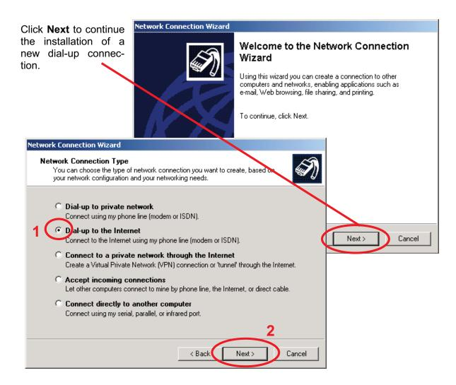
Tap **Dial-up to the Internet** (1) and click **Next** (2) to proceed with the installation of a new dial-up connection.
