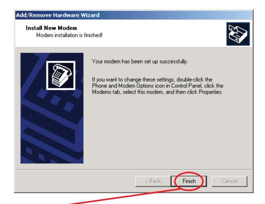
Click on **Finish** to terminate the modem installation.
